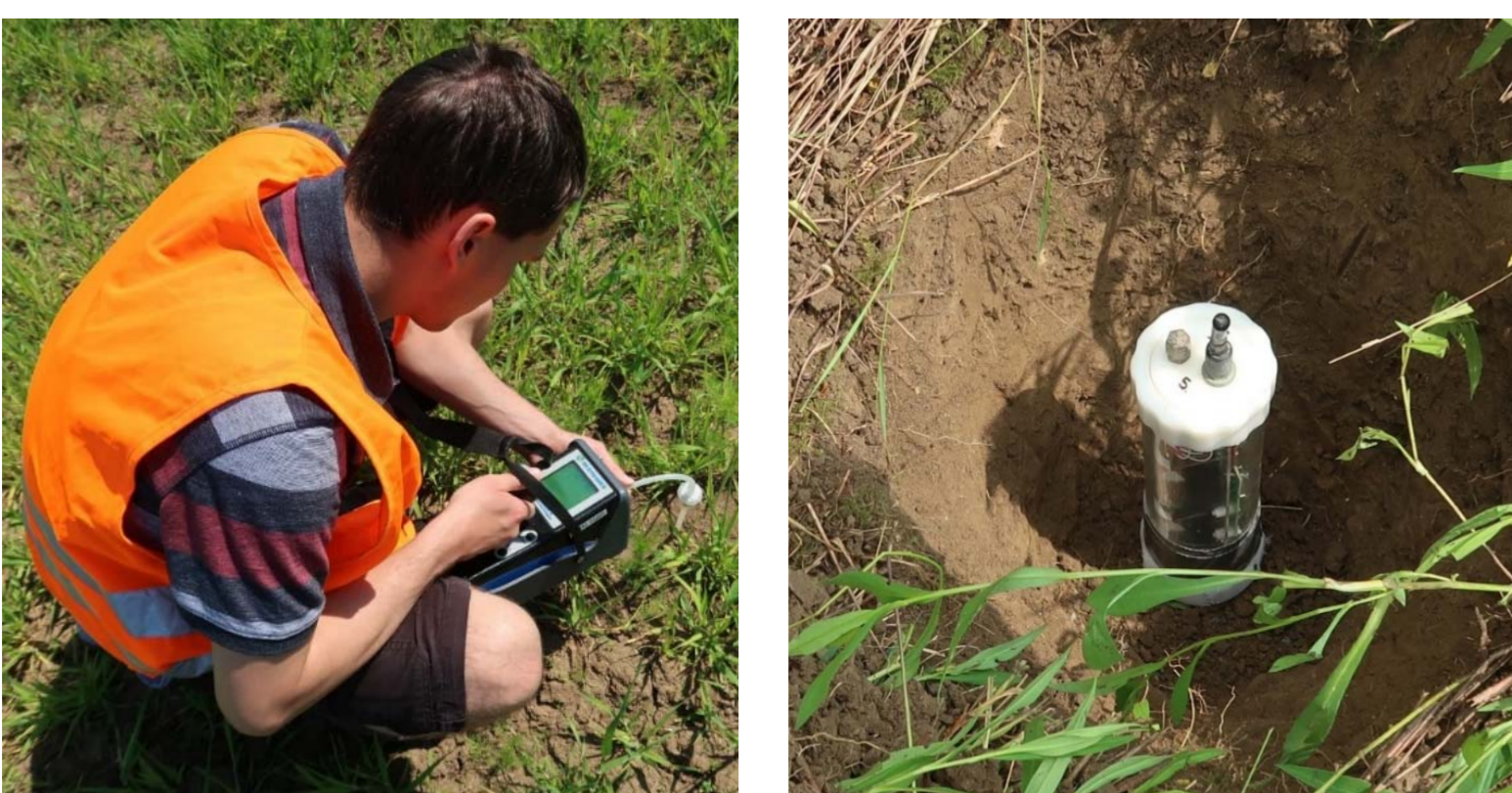
Periodical soil-gas monitoring using the Ecoprobe-5 (left) versus IGS permanent probe used for the continuous monitoring (right).
