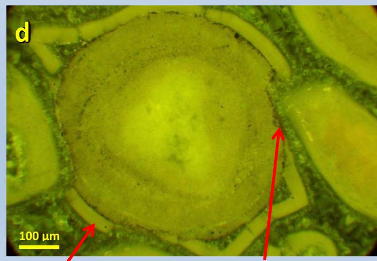
c-d): deformed ooid – the cracked micritic coating, pressure dissolution
