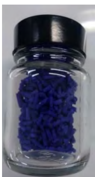
Figure 1: UTSA-16 extrudates used in this study.
