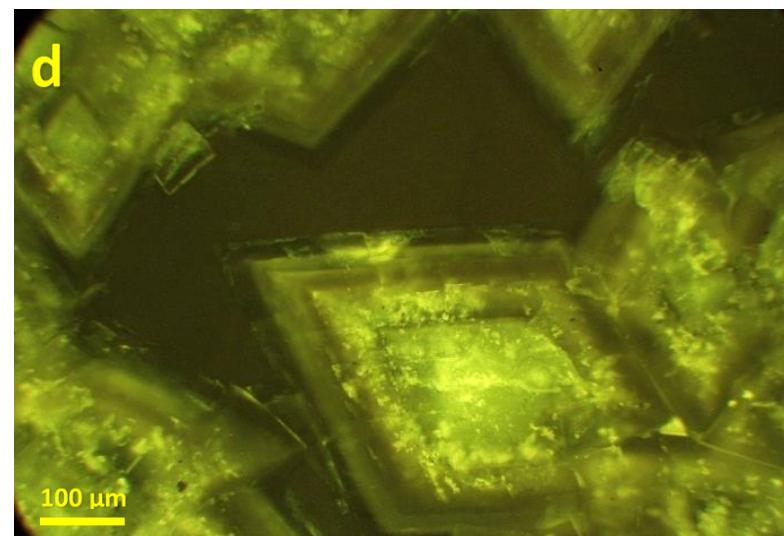
*pD – pore-lining dolomite (arrow in fluorescence light)*
