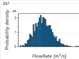
CO<sub>2</sub> leakage rate simulations per well
