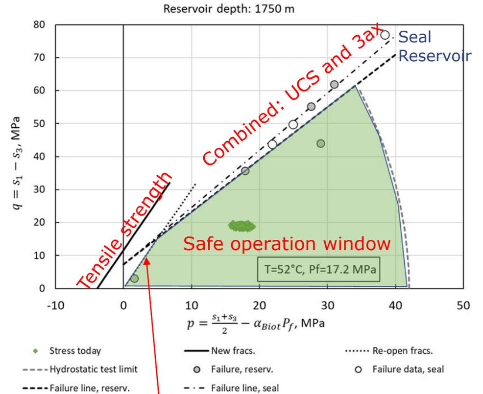
Re-open existing tensile fractures
