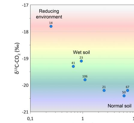
Carbon isotopic composition of  $CO_2$  ( $\delta^{13}C$ - $CO_2$ ) shows more negative values with increasing CO<sub>2</sub> content in soil gas.
