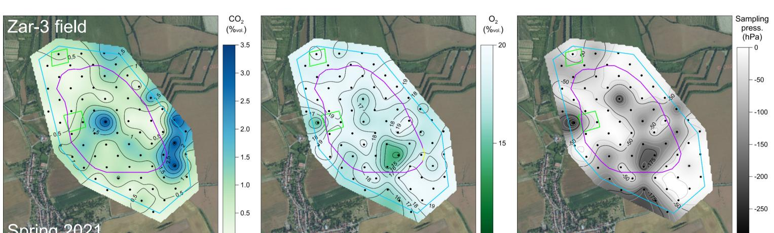
Contour maps of the average CO<sub>2</sub> and  $O_2$  content in soil gas (both in  $%_{vol}$ ) and sampling pressure (hPa) in spring 2021. Effects of land use - field ploughing - is clearly visible in SE part of the monitored area.
