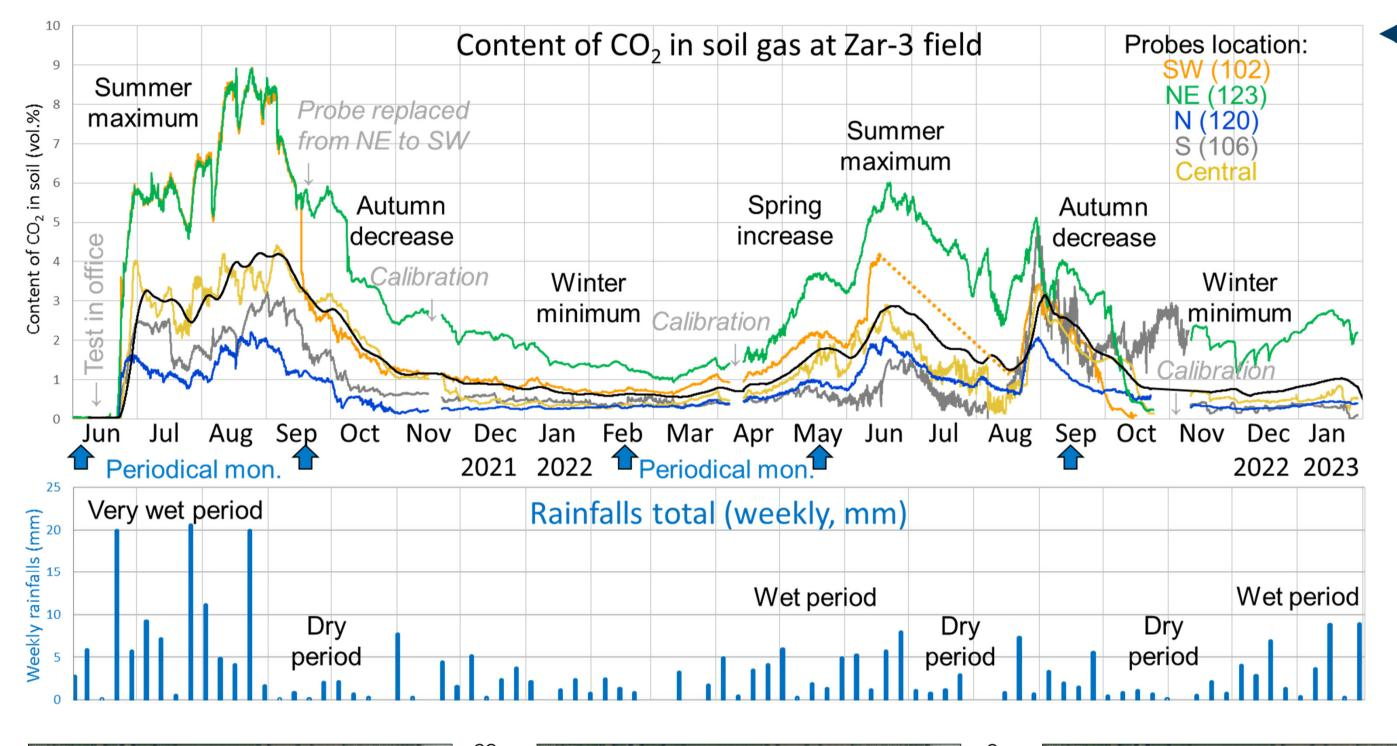
**◄** Time-plot of CO₂ content in soil gas measured by five permanent probes (in colors) related to the rainfalls total (bottom). Maximum CO<sub>2</sub> content in soil gas was measured in summer seasons and during and after strong rainfalls.
